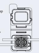
5. Using 8"-10" Straight Jaw, Groove Joint Pliers, individually press blade holders into housing until blade holder is fully seated in housing. Verify top surface of blade holder is even or just below the top surface of the housing.
