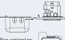
4. Place unstripped tap conductor into side B (see image in step 2). Insert conductor until visible against stop on opposite side.
